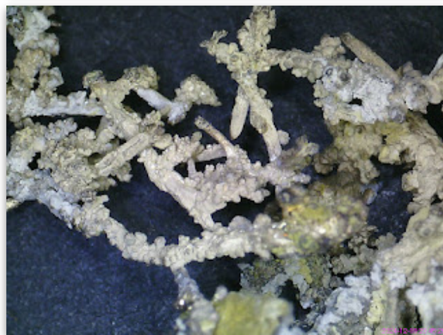
Above: Wire silver covered with small nodules of acanthite (silver sulfide) and chalcopyrite (copper-iron sulfide). Collected from the Last Chance Mine. Width FOV ~6-7 mm. Photomicrograph: M. Nelson
